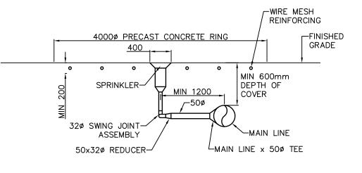
SPRINKLER DETAIL SCALE: NTS
