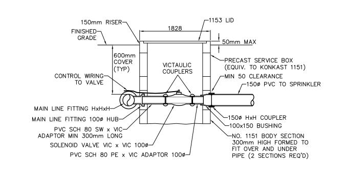
SOLENOID VALVE AND ENCLOSURE DETAIL SCALE: NTS
