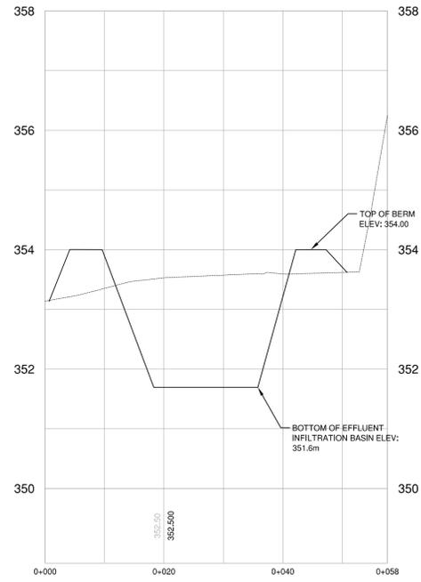
**C EFFLUENT INFILTRATION BASIN SECTION C-C**
