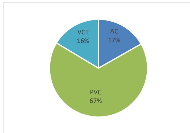
**FIGURE 5-6: COLLECTION NETWORK PIPE MATERIAL PIE CHART**
