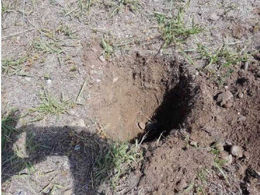
**Photo 9:** Soil pit on proposed irrigation area at airport. At this location, a residual A/Ap horizon is present. Note fine roots in upper 10 cm.
