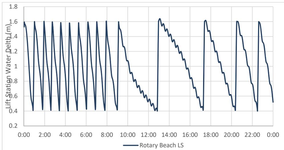
**FIGURE 5-5: PCSWMM RESULTS – ROTARY BEACH LIFT STATION DEPTH**
