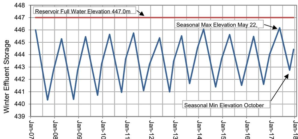
FIGURE 4-1: RESERVOIR WINTER EFFLUENT STORAGE ELEVATIONS (2005-2017)
