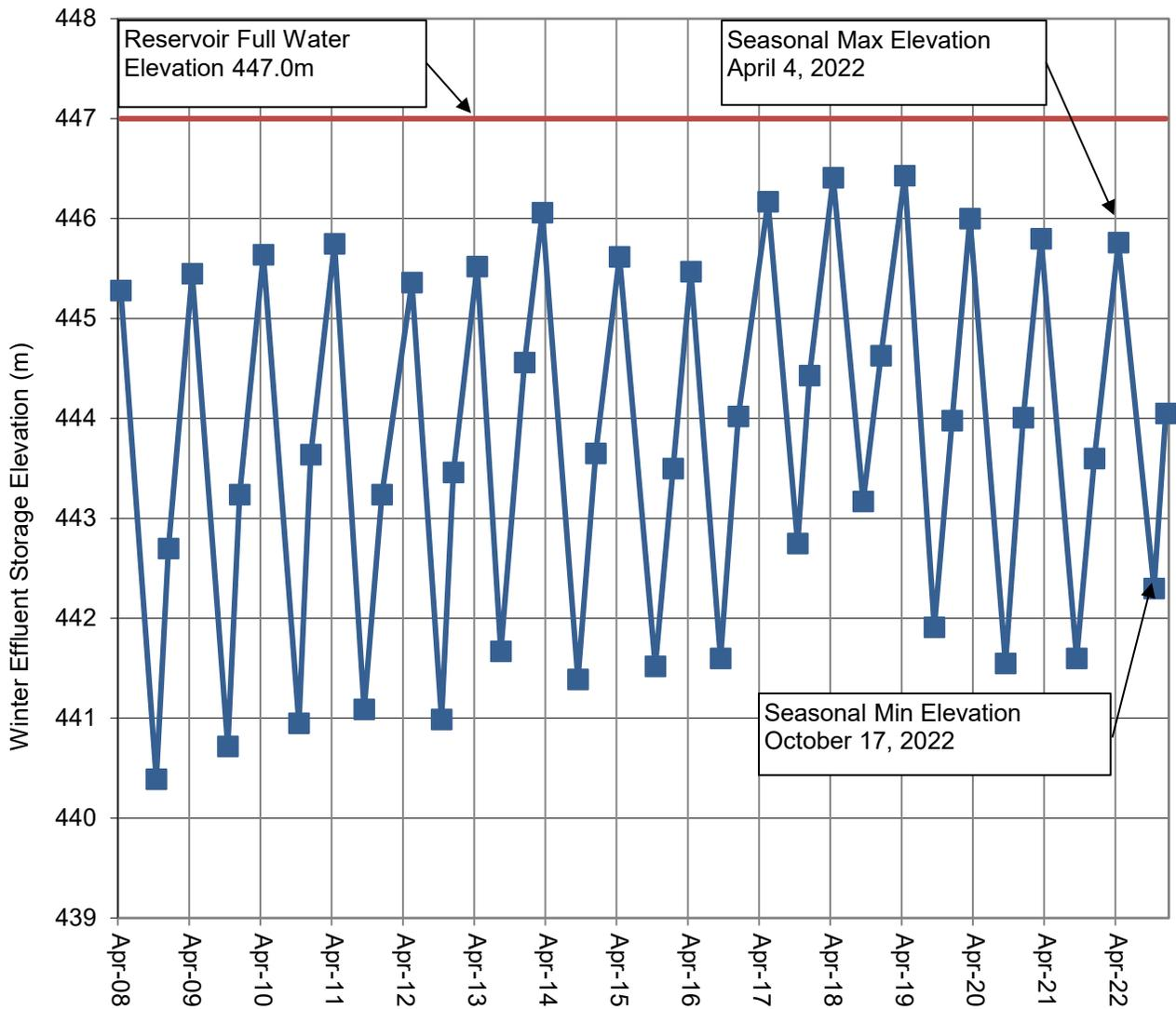
FIGURE 1-5: EFFLUENT STORAGE RESERVOIR LEVELS - 2008 TO 2022
