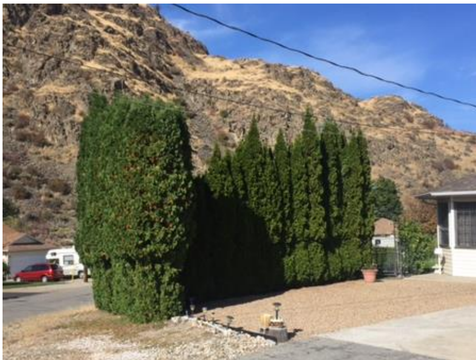
FIGURE 13. Although there is some separation between the cedar hedge and the home in this photo, the hedge is likely still too close. If the hedge were to catch fire during a wind-driven fire, flames could impinge on the adjacent window, siding and eaves of the home.
